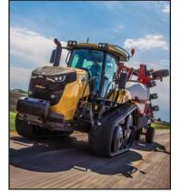
the CVT, PTO, cooling system, and hydraulics, are geared to run at optimum levels at this low engine speed. This delivers lower fuel consumption, reduced engine and component wear, and quiet operation. The three-stage Maxx Ride<sup>™</sup> Integrated Comfort System (ICS) delivers a quality ride. The system is comprised of a redesigned oscillating midwheel system, all new primary hardbar suspension, and advanced cab suspension.
