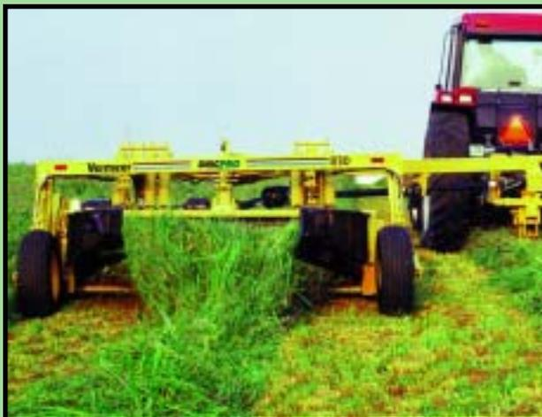
The Vermeer DiscPro Mower Conditioner is a new concept in domestic mower conditioners. One feature that sets the DiscPro apart from other machines is its swing back suspension, which swings away from obstacles in its path. The suspension minimizes lifting force through its range of motion. Other machine suspensions push their headers from behind with suspension arms angled down. When the headers strike an obstacle, they are forced into the ground, which causes undue stress to the machines.
