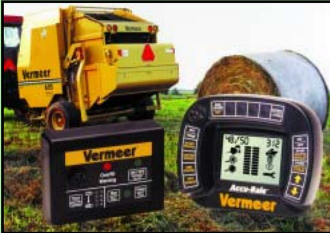
The Accu-Bale control system for round balers consists of a controller, wire harness and sensors mounted on the baler. The controller displays bale size throughout bale growth, plus bale shape, bale count, tailgate status, tie/wrap cycle status and error messages. The system allows tractor seat operation of bale size setting, twine or netwrap selection, twine or net applied amounts, miscellaneous tie/wrap cycle modifications and volume level.
