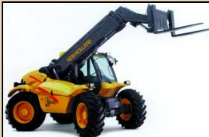
The Model LM430 Telehandler is a new materials handler for the agricultural market. It features a 106-hp engine and two-section telescoping boom that extends to 22 ft. (6.6 m) for improved reach and lift. A hydraulic joystick controls boom movement.
