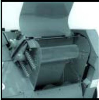
The New Holland CropPro™ crop processor attachment chops and processes corn silage in one operation with a pull-type harvester. Mounted above and behind the cutter head, the CropPro cracks and crushes corn kernels while shearing and crushing stems and cobs. This system eliminates the time and expense of using a stationary roller mill.
