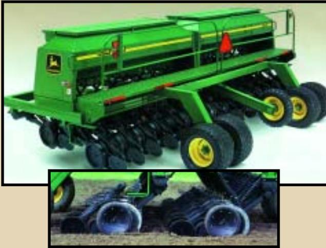
The John Deere 1560 No-Till Grain Drill incorporates customer requests such as a patented feature that allows the opener to float over undulating soft soils for increased depth control without excessive down force. Opener down force is adjusted hydraulically to match field conditions from a single point by 0.25-in. (0.63-cm) increment depth settings from 0.5 in. (1.27 cm) to 3.5 in. (8.9 cm) No tools are needed for depth adjustment or down force settings.
