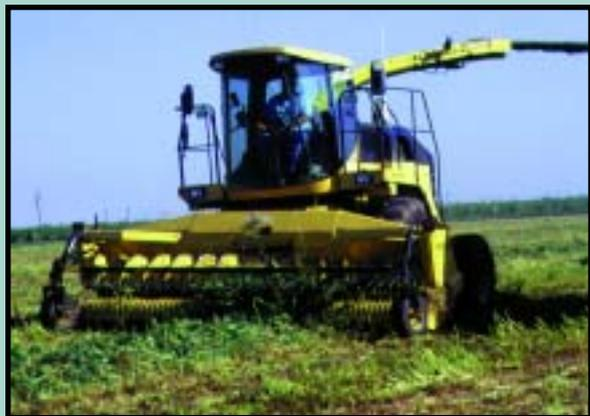
New Holland's extra-wide Model 365W Windrow Pickup Attachment harvests volumes of crops quickly, its 15-ft. (450-cm) pickup handling bigger, wider windrows. It picks up two windrows at once and sweeps field corners for complete pickup in one pass.
