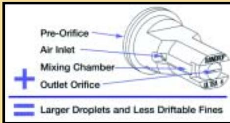
A RAINDROP® ULTRA nozzle includes a round pre-orifice to meter fluid, an elliptical outlet orifice to form a fan spray and a mixing chamber between the two. The mixing chamber is vented by two side holes near the pre-orifice. A high velocity jet from the pre-orifice causes a vacuum zone near the side holes and air is induced into the mixing chamber. Air and liquid mix in the chamber and axially travel toward the elliptical outlet orifice.
