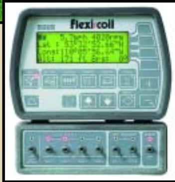
The Flexi-Coil Task Controller allows automated variable rate application of seed, fertilizer or herbicides using GPS control. The Task Controller uses location information from the GPS receiver to adjust rates via FlexControl electronics according to information supplied by the farmer.
