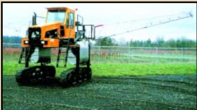
Twelve-inch-wide (30.5-cm) tracks and 65-in. (165-cm) ground clearance make the self-propelled, hydrostatically driven, rubber track GK TR4 Track sprayer suitable for a wide variety of row and field crops. With 5.4-psi ground pressure, growers can spray when it is too muddy for traditional wheeled sprayers. The TR4 rides and handles smoothly using a bogey roller suspension system on the tracks and an adjustable steering wheel control inside a reversible cab to suit field conditions.
