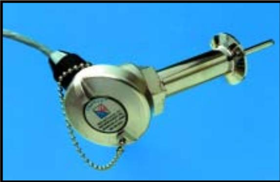
The FiberView sensor measures light backscatter — light reflected off particles in the opposite direction of incidence. Light from an LED is transferred to particulate fluid through optical fibers and transmitted back to a detector.
