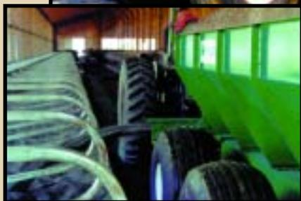
The McLanahan Stall Filler reduces time for adding bedding sand to dairy freestalls. The Stall Filler is towed into a barn and evenly distributes sand down the row of stalls. A sand hopper is mounted on a heavy-duty steel frame with a tandem walking beam suspension system. High flotation tires safely distribute the weight of a fully loaded Stall Filler as it moves over concrete.
