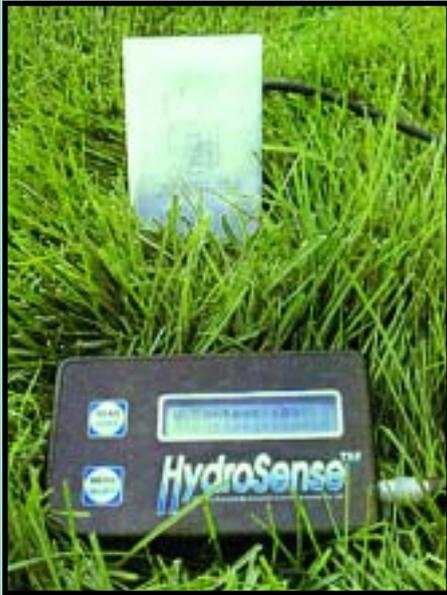
The portable HydroSense™ Soil Water Measurement System consists of a digital display and probe easily inserted into the soil surface. The system's water content measurement mode displays volumetric water content in percentages. The water deficit mode displays a relative water content based on user-chosen lower and upper water content reference levels. The device also displays the amount of water needed to bring the water content to the upper reference value.
