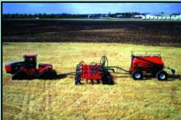
The AFS Concord Air Seeder provides an integrated system for controlling seed, fertilizer and anhydrous ammonia application from an in-cab display unit. Besides application rates, the system controls and monitors the hydraulic fan. It also monitors individual run blockages and product status can be viewed through a four-level bin sensor system.
