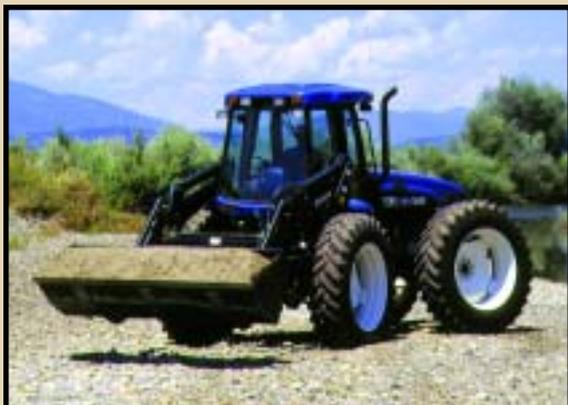
The New Holland Model TV140 Bidirectional™ Tractor can be operated engine-end or cab-end first to provide maximum productivity and loader performance. The redesigned 105-hp machine features a PTO and 3-point hitch at both ends for double capacity to mow, condition, till, plant, cultivate, spray, or push and pull mowers simultaneously.
