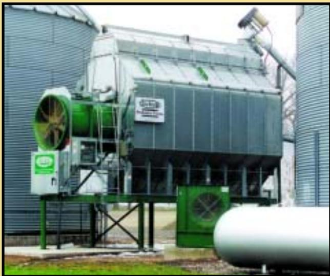
The Sukup Automatic Grain Dryer's main feature is its patent pending quad metering roll system. This system produces more even moisture content as its upper metering rolls move the hotter, inner layer of grain down the dryer column faster than the cooler, outer layer. The process reduces over drying and produces higher quality grain.
