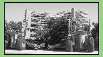
typical handpicking rate is 55 man-hours per semi-truckload. A pair of OXBO Citrus Harvesters is capable of reducing manpower to three to six hours per semi-truckload. This is an average labor productivity increase of 900 percent.
