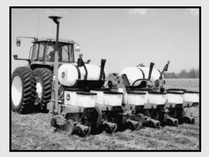
marker arm. The machines plant in all field conditions such as conventional till, mulch till and true no till. They are equipped with MaxEmerge<sup>®</sup> Plus row units, which provide high strength, depth control and seed spacing. A new mounting bracket which allows the use of John Deere frame-mounted fertilizer openers is also available.
