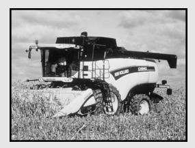
pressure compensation modes. The CX rear-axle design allows the rear wheel to tuck forward for a shorter turning radius and maximum productivity.
